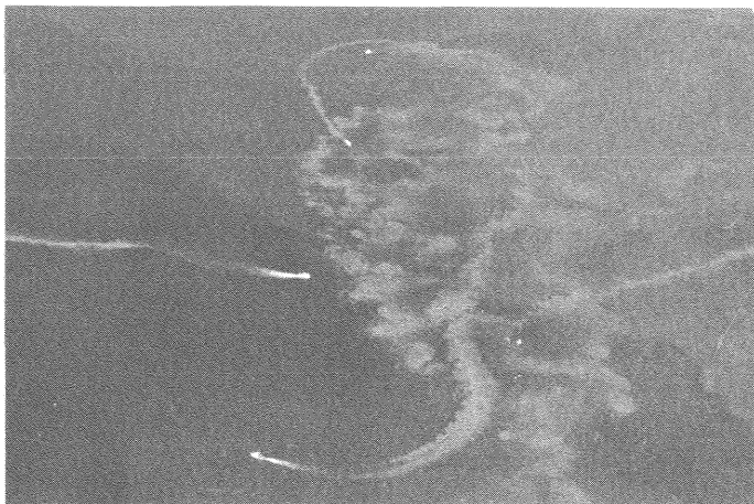
Aerial view of shrimp boats in Corpus Christi Bay (Texas) showing trails of sediment suspended by their weighted nets. MSRC scientists have shown that each year shrimpers resuspend 10-100 times as much sediment as is dredged for channel maintenance.
